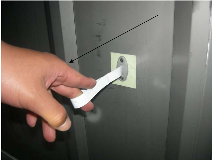
Emergency pull fitting, pull emergency pull tape to open lock handle bracket for right door leaf
