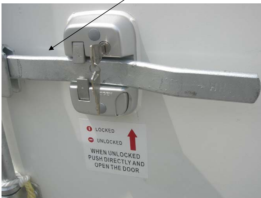
Locking handle bracket with locked by key that right door leaf can not be opened.
